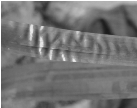
图6 喷油互感器解体顶部绝缘虚软空穴 Fig. 6 Virtual soft void on top insulation after disassembly of the oil injected current transformer
