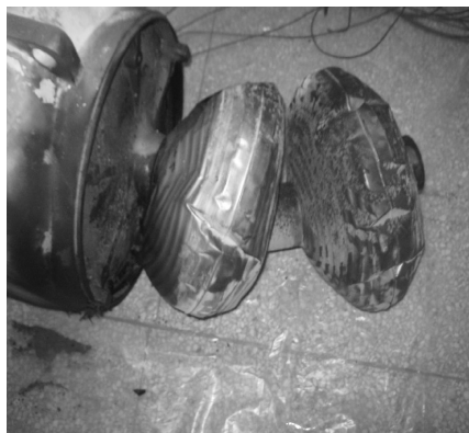
图5 电流互感器膨胀器撕裂喷油 Fig. 5 Torn and oil injection of current transformer expander
