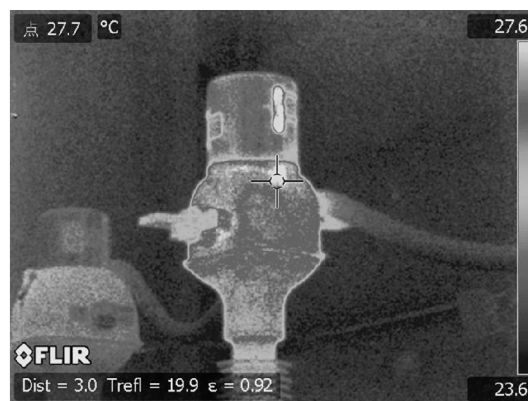
图12 长时加压两互感器红外测温结果对比 Fig. 12 Comparison of infrared temperature measurement results between two current transformers under long-term voltage stress
