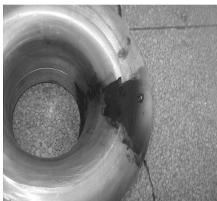
图4 铁心罩壳发生放电击穿 Fig. 4 Discharge breakdown of iron core casing
